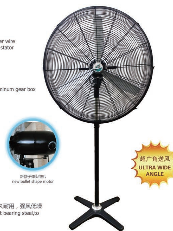
新款子弹头生铁圆形机壳 new-design bullet shape round cast iron motor housing 铝牙箱铁齿轮 aluminum gear box and iron gear wheel 电木开关 bakelite switch 新款铝板大三叶 new-design big 3 aluminum blade 2.0mm线径8mm间距 16根扁线自扣网 2.0mm wire diameter and 8mm wire spacing ,16 pcs , clip type fastener grill 1.3米伸缩杆 1.3m adjustable pole 7公斤十字铸铁底座 7kgs cross iron base
